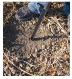
Taking a soil sample with an auger.
